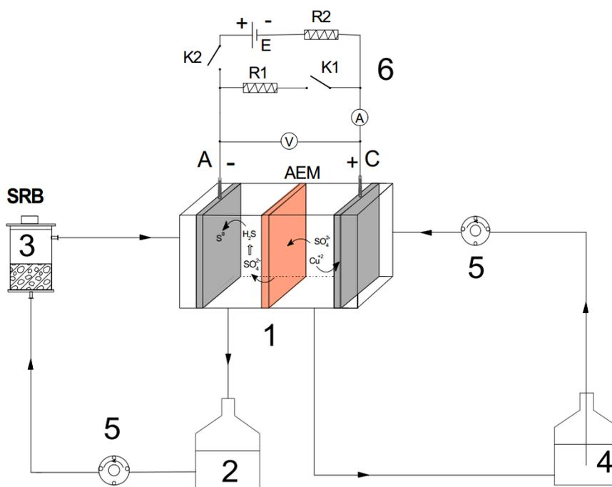
**FIG. 3.** Technological scheme of the laboratory installation under Variant 2
