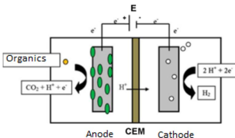
FIG. 1. Principle of operation of the microbial electrolysis cell (MEC)
